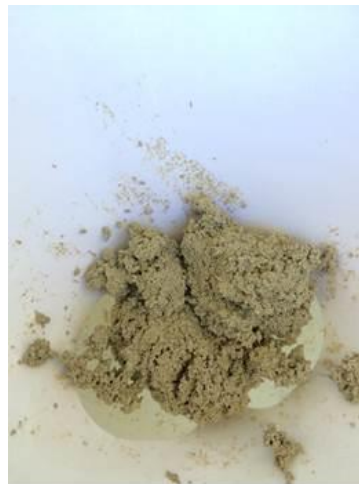
Figure 6. The dried paint slurry after sitting outside for 3 days
