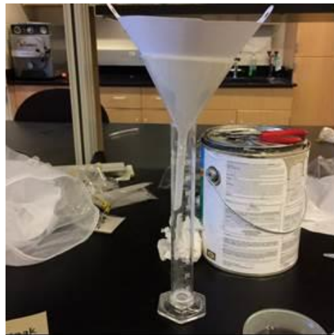
Figure 4. The filtration apparatus to measure leaching
